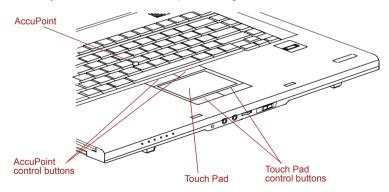
Figure 4-1 Touch Pad and Touch Pad control buttons
